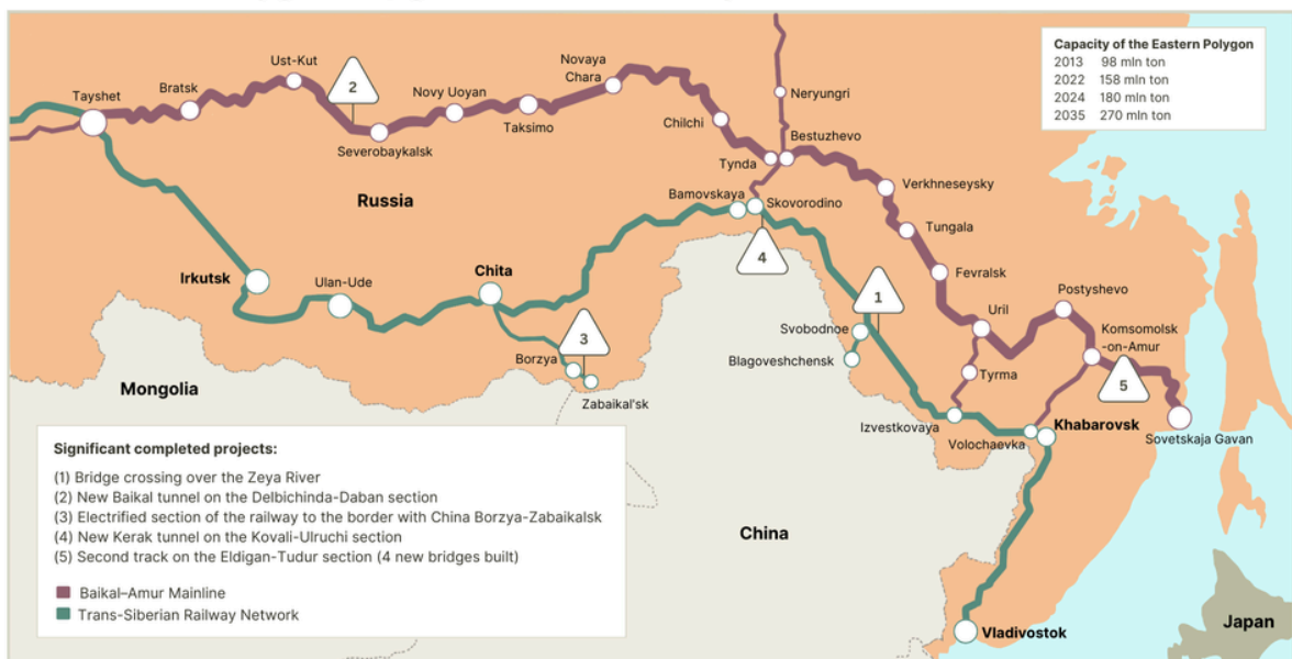
Figure 6. The Eastern Polygon - upgrades to the railway infrastructure
